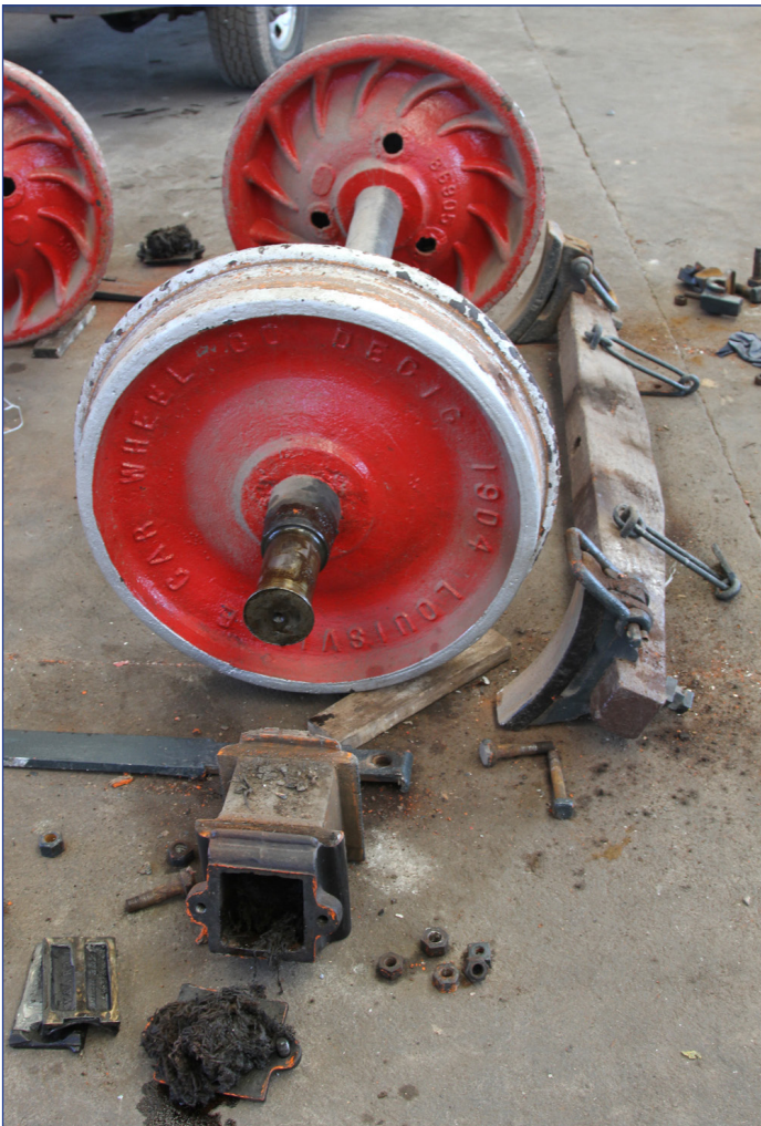
The Texas was rebuilt over a century ago by then-owner Nashville, Chattanooga, and St. Louis Railway prior to its donation to the "Ladies of Atlanta" - 1903 and 1904 tender wheels from that restoration lie next to their brake beam.
