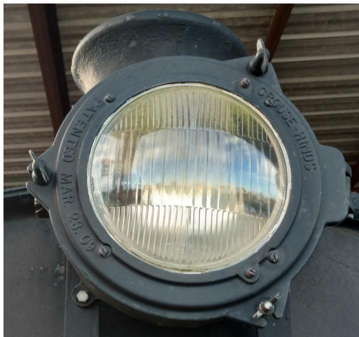
No. 7's Crouse-Hinds headlight casting has a patent date of March 23, 1909.
