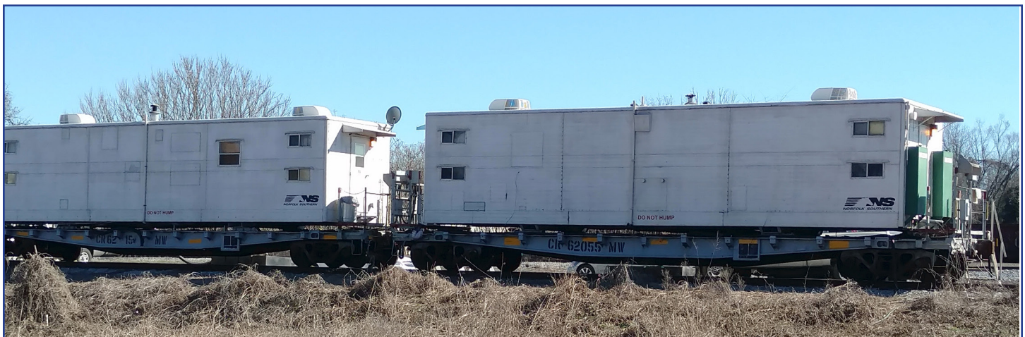
CR 6215? and CR 62055. A couple more notes for modelers: the green vertical tanks on either side of the doors are fuel tanks, the lights are on even when nobody is home, the bunk cars have at least two roof-top RV- style air conditioners, and most of the cars have satellite dishes...
