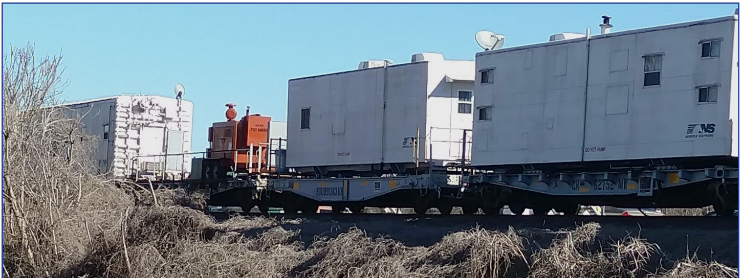
Left to right: a converted box car; a generator flat; a shorter flat and module, Southern 991353MW; CR 62752MW.
