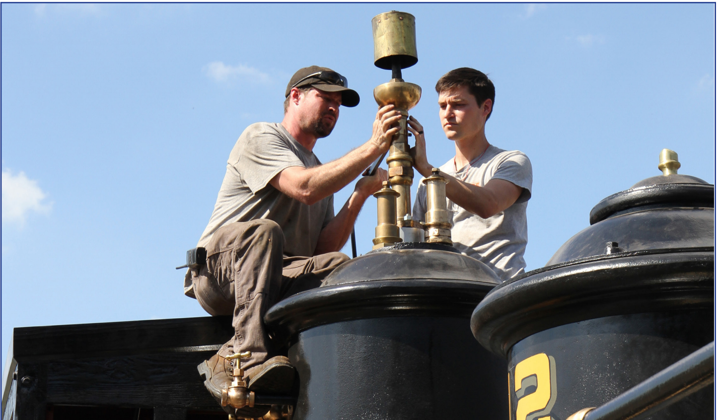
Nathaniel and Max adjust the whistle to operate on the roundhouse's compressed air.
