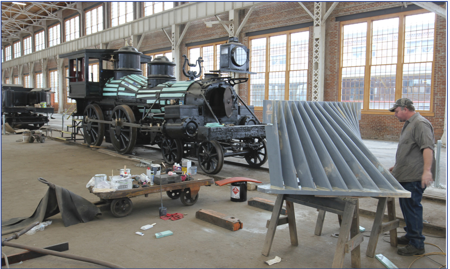
Eddie Mooneyham of SOC took a break from working on 611 to sand the new oak pilot. The Texas has yet to receive its new jacket.
