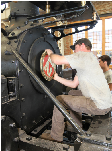
SOC craftsman Nathanial Watts applies the new No.12 number plate to the smoke box door. Nathanial came up with very effective "Russian Iron" jacket paint.
