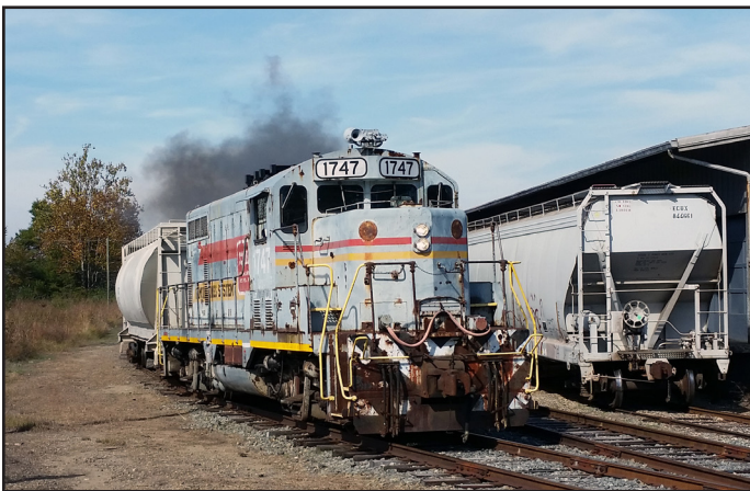
The Caldwell County Railroad exercised its former Family Lines GP-10 # 1747 in Hickory on October 28... the unit normally serves as a backup to GP-10 # 1811, which started life as ACL #111. Both units began life as high-nosed GP-7s.
