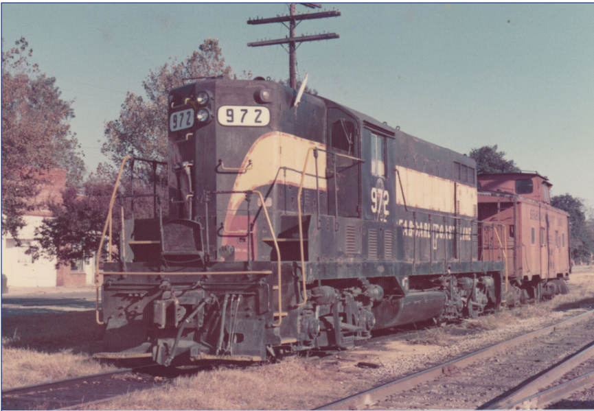
Seaboard Coast Line EMD GP-7 No. 972 was completed in February 1952 for predecessor Seaboard Airline Railroad as its number 1792.
